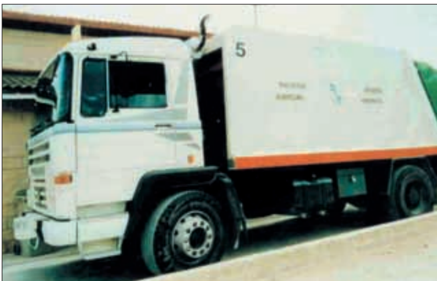
Above: House-to-house collection vehicle
